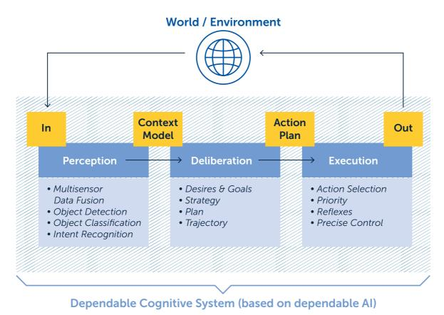
*Figure 1.* Sense-plan-act loop of a cognitive system.
